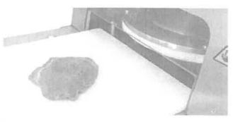
The MAGA® Meat Press automatically starts the flattening process when the tray is inserted.
